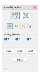
Select a part by clicking on the model. Move the cursor onto a part of the model in the display and move the part while pressing the left mouse button. In this mode only single parts can be moved.
