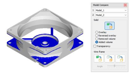
In this mode the models to be compared are put on top of each other in solid render mode.
