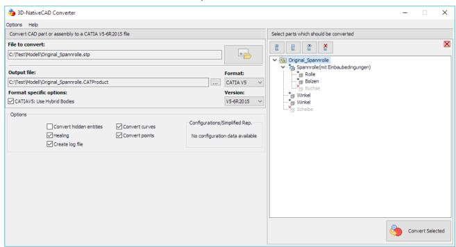
The assembly structure of the file to be converted will be read. For complex assemblies this may take some time. When the assembly structure is completely read, the Model Tree is displayed to Select *the parts which should be converted*.
