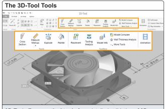
3D-Tool offers **practical tools** for a detailed validation of 3Dmodels: besides measure and analyzing tools also a Model Compare and tools such as Painter, Explode and Animation.
